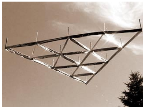
Scalability: Lifter technology becomes more efficient at larger sizes – this is the Lifter 4 outdoors during a July-2002 demonstration.
