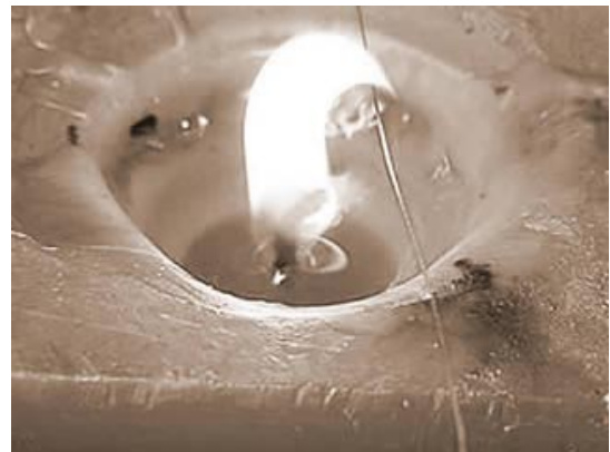
Atmospheric Plasma: A candle-flame burning against gravity due to a high-voltage plasma interaction.
