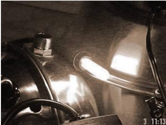
UV Bulbs: Germicidal bulbs produce ionizing UV and are used in water-treatment.
