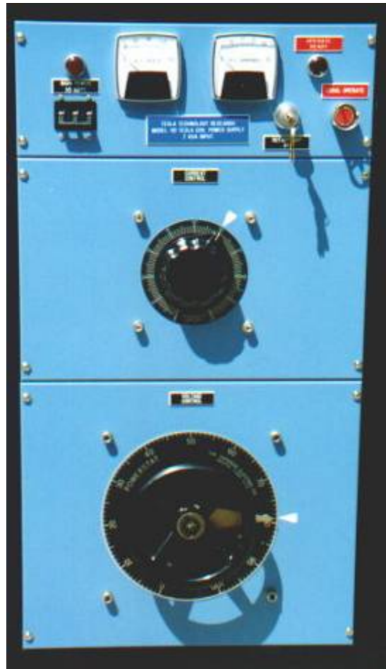
Power-Supply: A closeup for a high-output power-supply to drive a resonant coil system.
