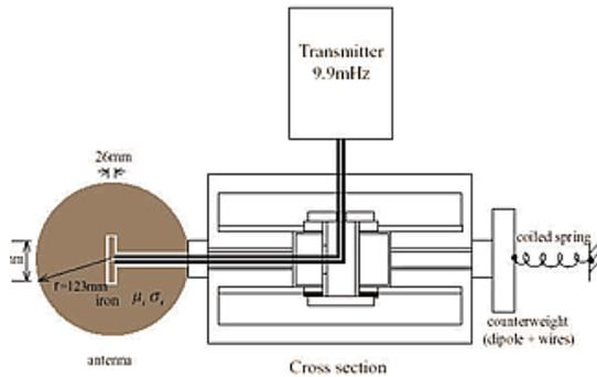
**Sys-H Assembly:** De Aquino provided this system-prototype design schematic.
