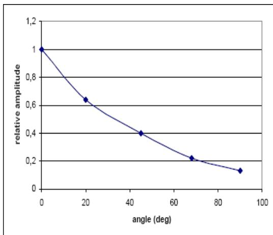
**Deflection:** Angle of pendulum deflection correlated with adjusted pulse amplitude.
