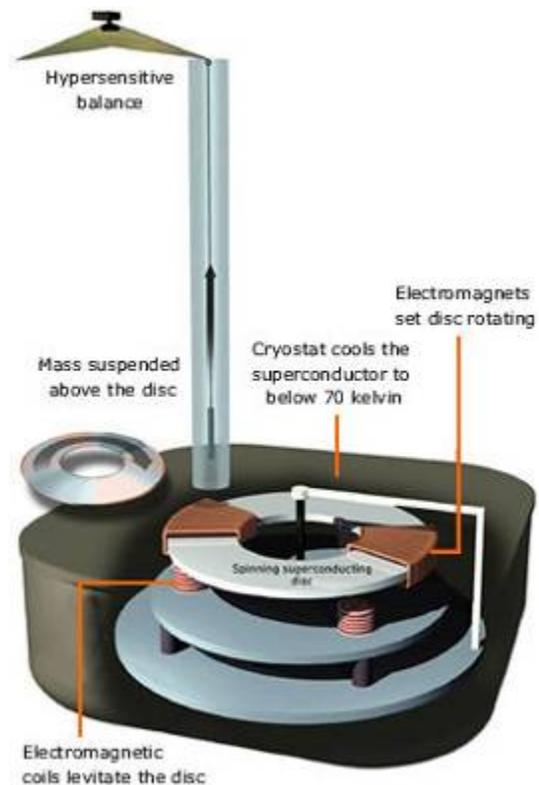
**Rotating Disk:** A cutaway of the Type-II disk apparatus from the first experiment.
