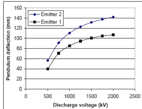
**Deflection:** Deflection of pendulum during testing as a function of discharge voltage.
