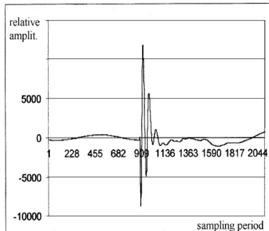
**Amplitude:** Relative pulse-amplitude from impulse-discharge experimental testing.
